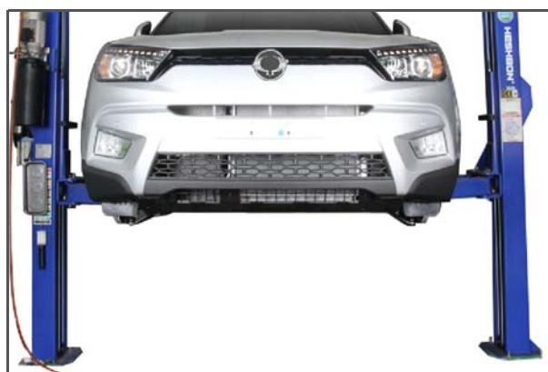
When working on the vehicle using a lift, do not run the tires with all the wheels off the ground and the parking brake applied, as this may damage the E-coupling's clutch.
